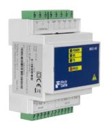
The electronic meters provide pulse output proportional to the energy measured. **MIO 40** is a centralized energy meter with four inputs (optocoupled) for reading these pulses. Their values are then stored on the memory.
